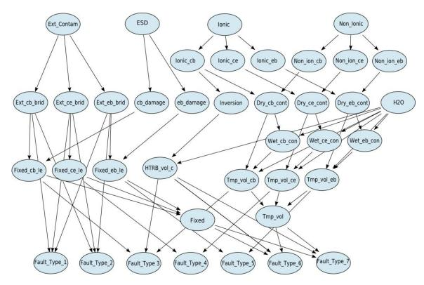
Figure 2. A Bayesian belief network representing the causal relationships and data points implicit in the discrete component semiconductor domain. As data is "discovered" the (a priori) probabilistic hypotheses change and suggest further search for data.
