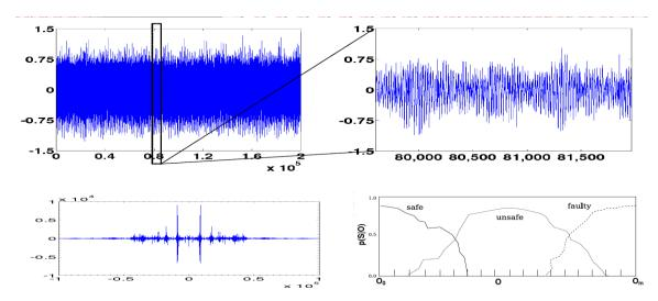
Figure 3. Real-time data from the transmission system of a helicopter's rotor. The top component of the figure presents the original data stream (left) and an enlarged time slice (right). The lower left figure is the result of the Fourier transform of the time slice data (transformed) into the frequency domain. The lower right figure represents the hidden states of the helicopter rotor system.
