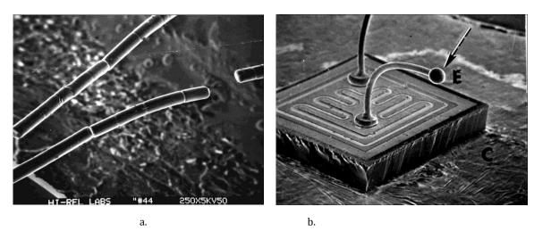
Figure 1. Two examples of discrete component semiconductors, each exhibiting the "open" or "connection broken" failure.
